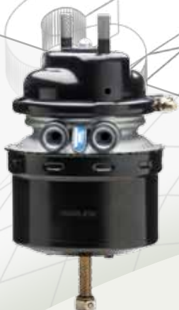
Cj Câmara Tristop Baioneta - Truck - Rosca M22 Voss / Tipo 16 / 24 P/ Freio a Disco | Câmara de Freno Bayoneta - Truck - Rosca M22 Voss / Tipo 16 / 24 | Bayonet Brake Chamber - Truck - Threaded M22 Voss / Type 16 / 24
